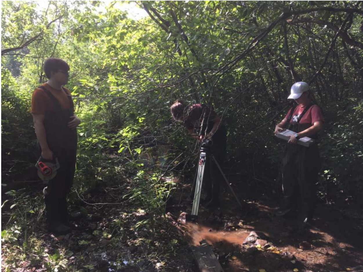
Figure 11: Field staff using automatic optical level to read levelling rod.
