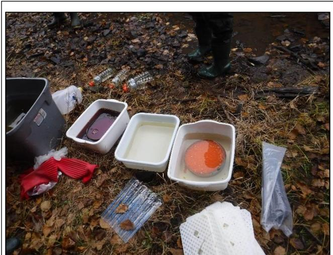
*Photo illustrating three stages of disinfection; Ovadine solution, rinse bin, fresh brook water*
