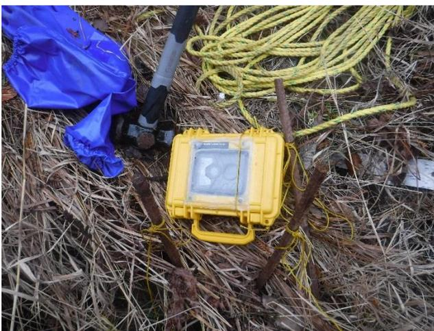
*Underwater camera unit with attached rebar*
