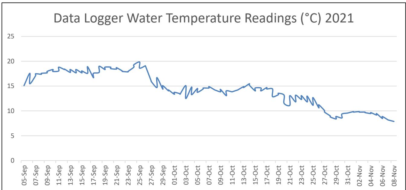
**Figure 3: ONSET water temperature data logger readout (12-hour intervals); channel shifting caused data logger to be closer to surface resulting in warmer temperatures, surface water temperature not representative of overall water column**
