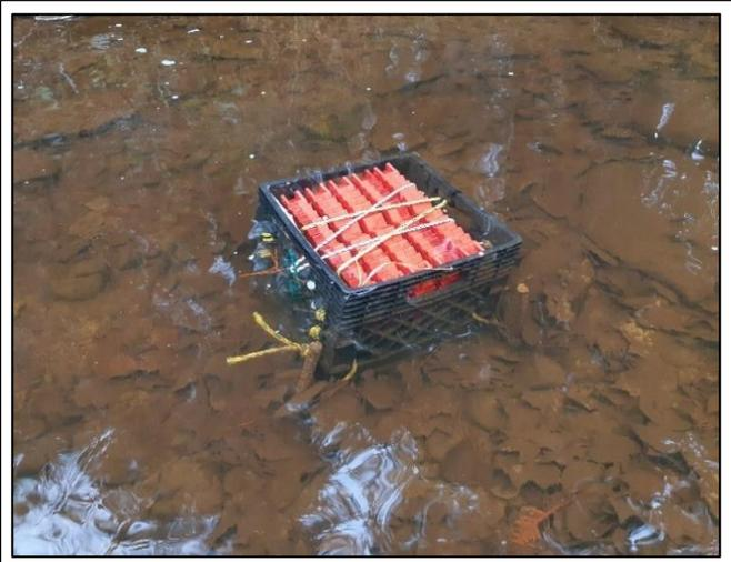
*Photo of milk crate design with loaded incubator installed*
