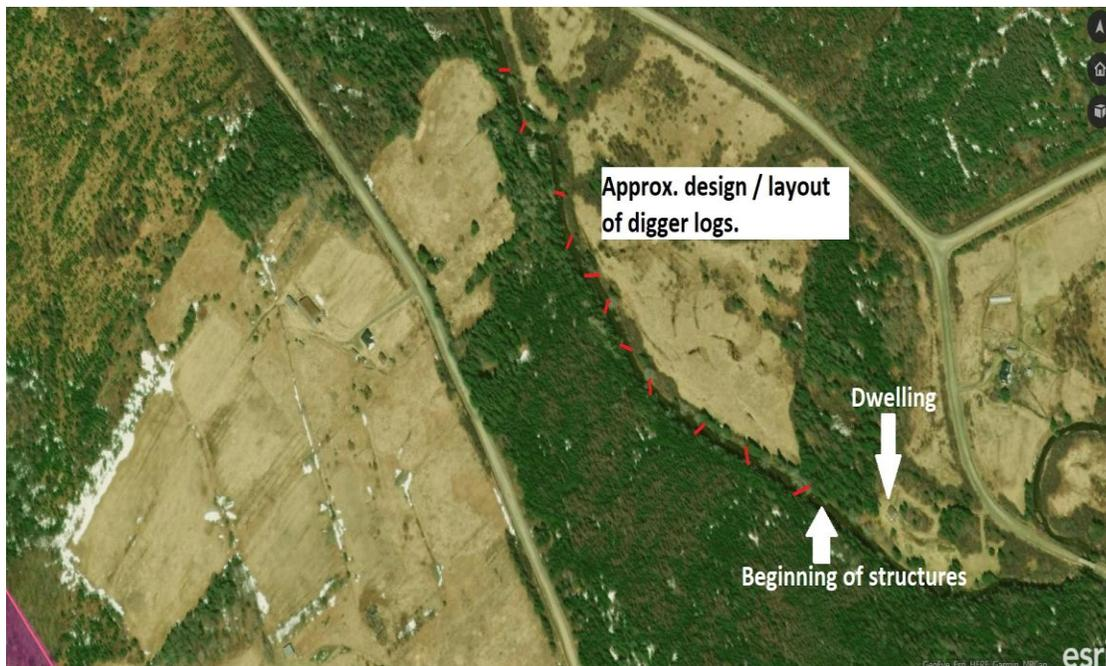
Figure 15: Red lines denote approximate location and design of digger log structures.
