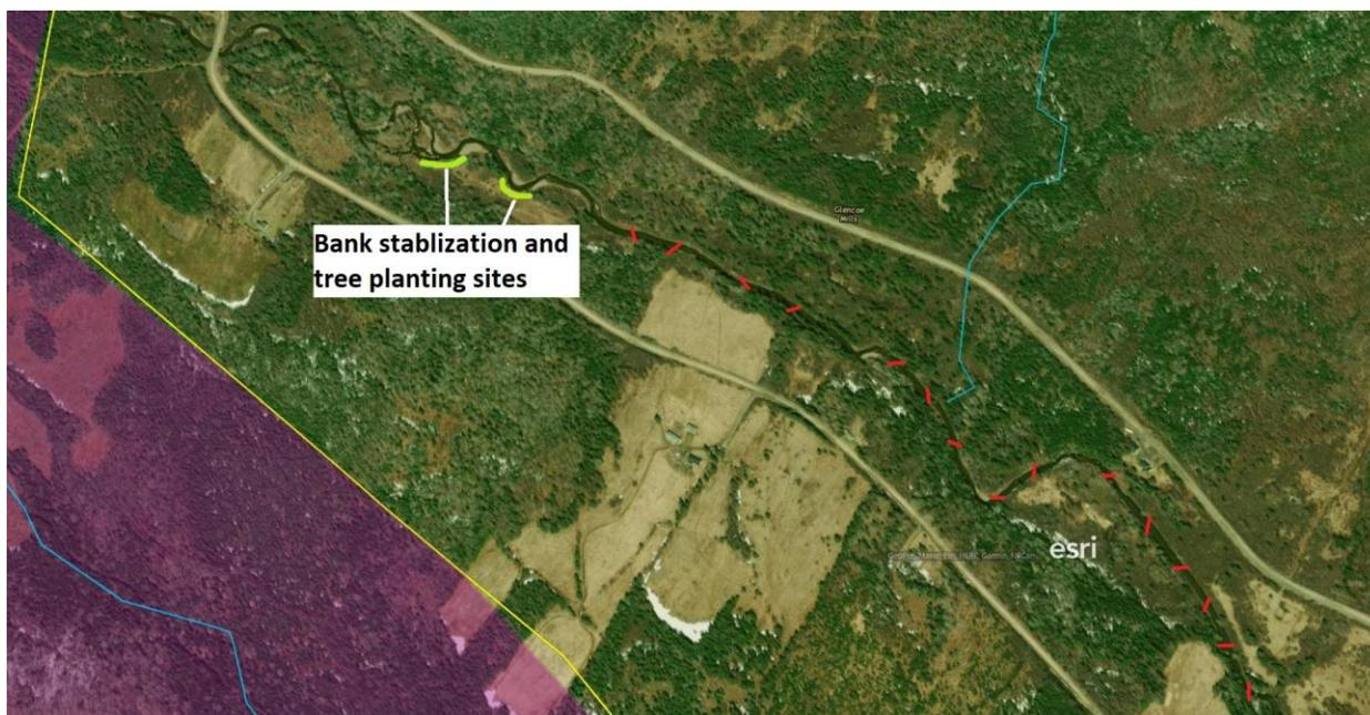
Figure 16: Approximate layout of instream restoration structures. Digger logs denoting in red.
