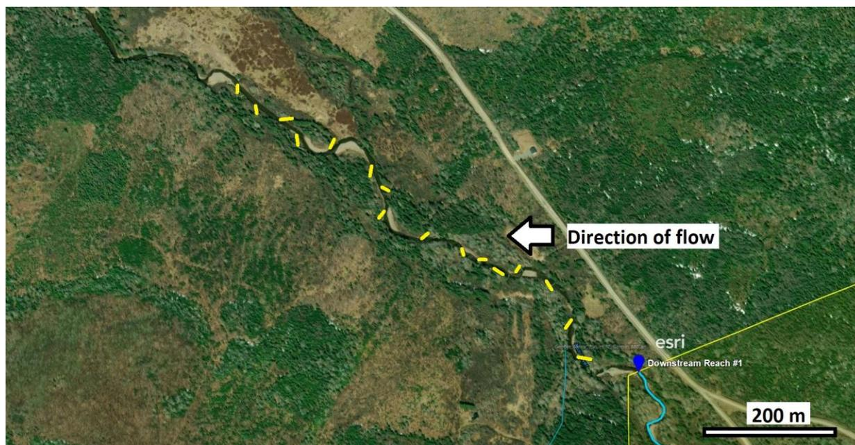
Figure 44: Approximate placement of deflector structures in upper section reach #2.
