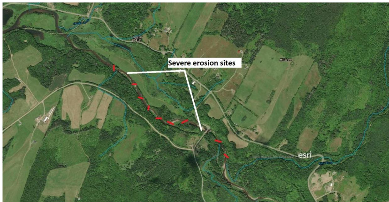
**Figure 73: Approximate layout of structures. Bank stabilization work will be required to address erosion issues.**
