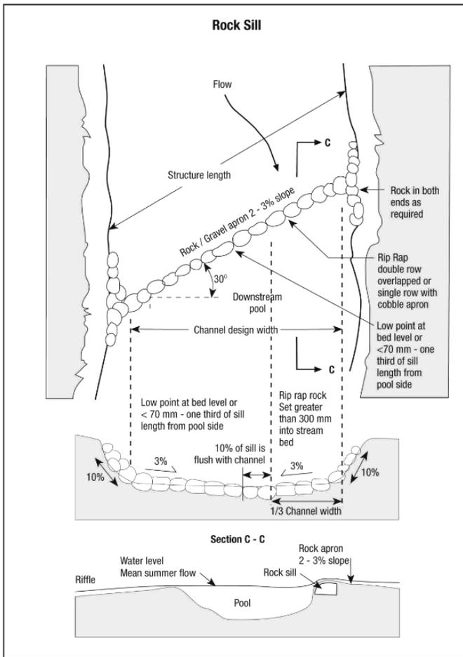
**Figure 6:** Basics of a rock sill used at the head of a pool.
