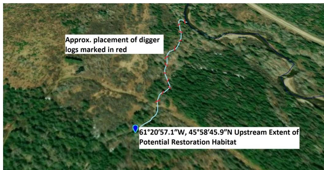
**Figure 41: Satellite image showing approximate location and sequence of digger logs.**
