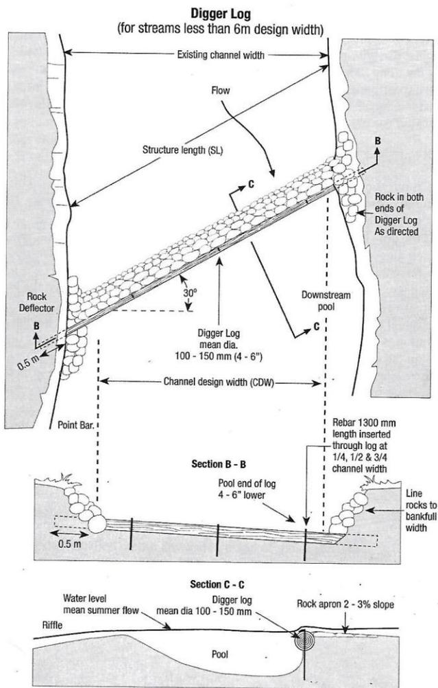
**Figure 5:** Conceptual drawing of a digger log
