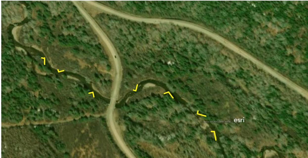
Figure 17: Lower sites on reach #1. Deflectors are most appropriate technique.
