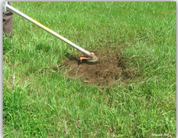
Figure 9.8 Hawk attachment on a brush saw for planting site preparation in grass
