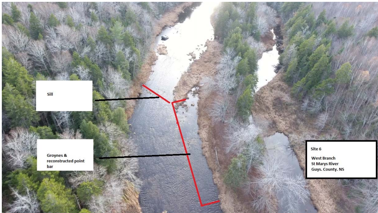
Figure 23: Conceptual design of restoration work on Site 6.
