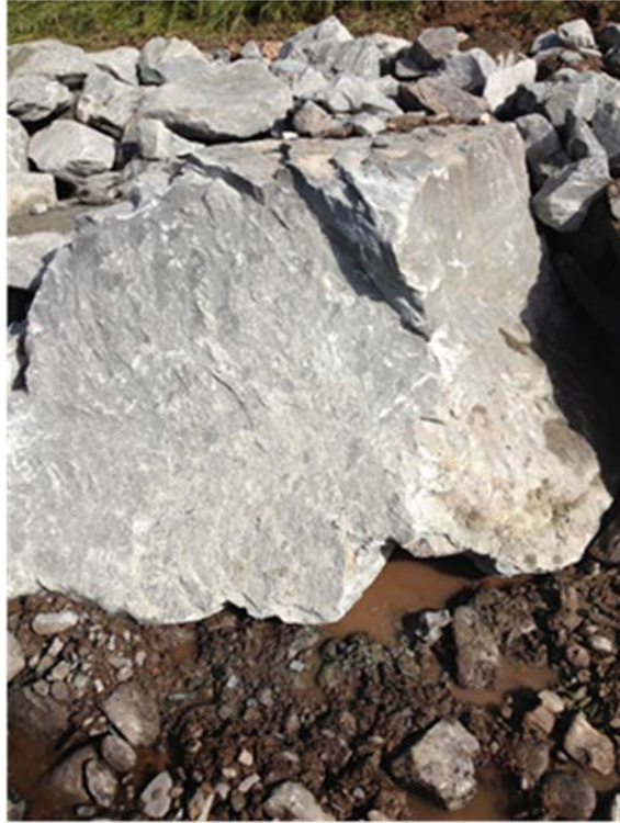
Figure 18: Example of two tonne rock used at Site 4 for bank protection.
